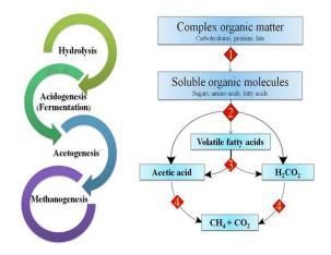
Figure 4. Stages of anaerobic digestion
