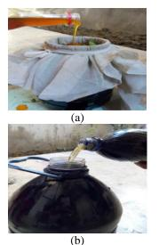
Figure 8. Anaerobic digestion (a) net bag (b) without a net bag
